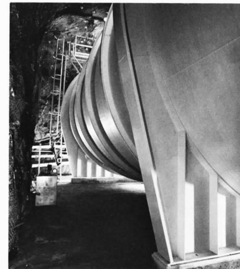
Fig. 3 Solar neutrinos are detected by this equipment in the Homestake Gold Mine, Lead, South Dakota (photograph by permission from R. Davis, Jr., Brookhaven National Laboratory).
