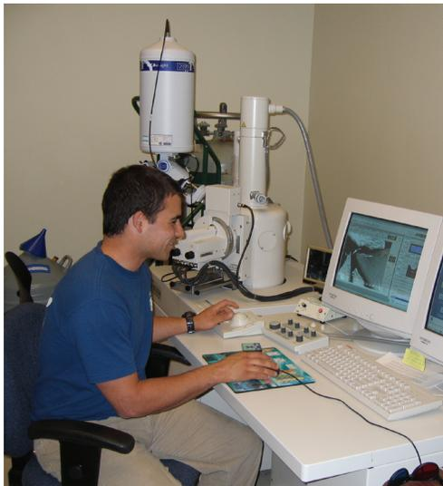
*Mark Wollam operates the Scanning Electron Microscope/Energy Dispersive X-ray Elemental Analysis System in the Keck Laboratory, part of the Cerent Engineering Science Complex.*
